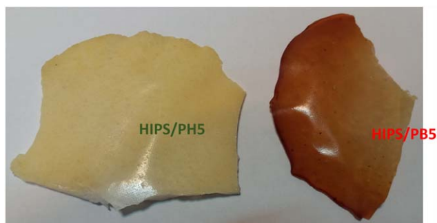
Figure 9. Color change of HIPS/PH5 and HIPS/PB5 samples after exposure to ozone and heat. [Color figure can be viewed in the online issue, which is available at wileyonlinelibrary.com .]
